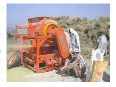
Machine was tested at three different threshing drums peripheral speeds; 500, 550 and 600 rpm for three crop moisture levels; 22%, 18% and 14%. Thresher performed best with speed of 550 rpm and crop mc 22%; at which threshing capacity was 372 kg per hour with threshing efficiency of 99.6% and fuel consumption of 4.6 litres per hour; while the total machine loss and seed damage was 0.3% and 0.2%, respectively.
